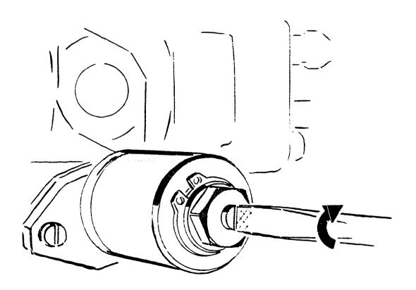
ADJUSTING SUPPLY PUMP PRESSURE AND TIMING-DEVICE TRAVEL
